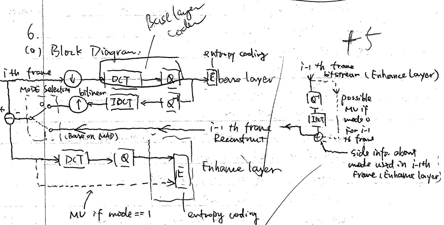
(\*) the above diagram omits some components in decoder of prediction loop
