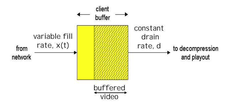
Client-side buffering, playout delay compensate for network-added delay, delay jitter
