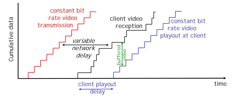
Client-side buffering, playout delay compensate for network-added delay, delay jitter
