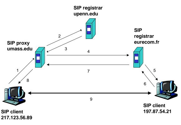
(4) umass proxy sends I NVI TE to eurecom registrar. (5) eurecom registrar forwards I NVI TE to 197.87.54.21, which is running keith's SIP client. (6-8) SIP response sent back (9) media sent directly between clients.
