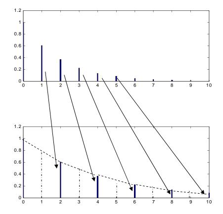
Missing samples need to be filled from neighboring available samples using interpolation filter
