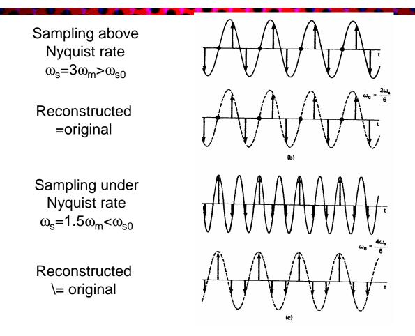
Aliasing: The reconstructed sinusoid has a lower frequency than the original!
