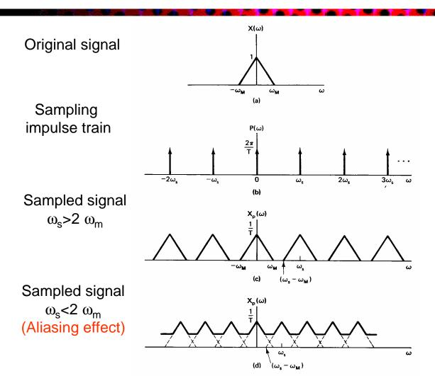
The spectrum of the sampled signal includes the original spectrum and its aliases (copies) shifted to  $k f_s$ , k=+/-1,2,3,...The reconstructed signal from samples has the frequency components upto  $f_s/2$ .
