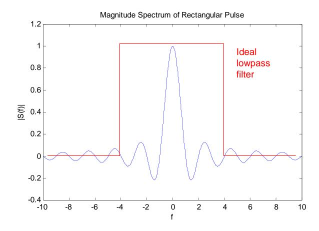
Filtering is done by a simple multiplification:
