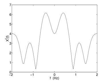
The frequency resolution of the DFT is the spacing between two adjacent frequencies:  $\Delta \omega = 2\pi/N$ .
