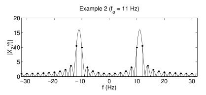
In Example 1, the DFT samples  $X^d(k)$  coincide with the nulls of  $X_2^f(\omega)$  and with its maximum value. In Example 2, they do not.
