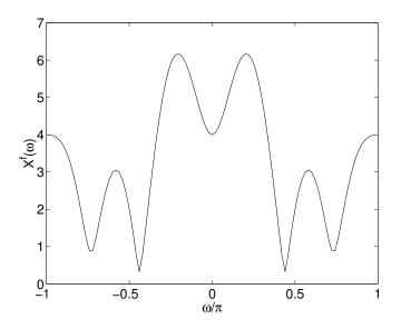
Then the DC component is in the middle of the spectrum. In Matlab, the command fftshift can be use for this.
