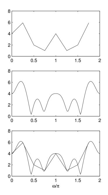
Zero-padding a sequence will result in a better plot of its DTFT. That is because the DFT samples the DTFT at the frequencies
