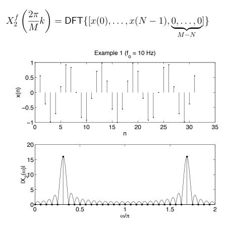
Lets use physical frequency with the DC component in the center.
