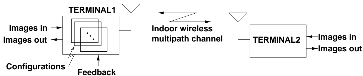
Figure 2: Indoor wireless image transmission system.
